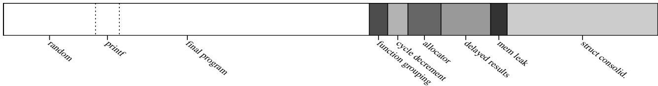
Figure 2. Run-time contributions of inefficiencies in the benchmark health. The shaded regions were optimized away through modifications of the benchmark’s source code. The white region corresponds to the final run-time, of which 25% is from the random number generator, and 7% is from printf s.
